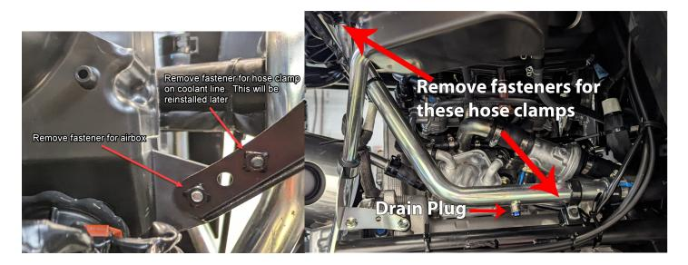
Shown here is one method of draining the radiator without making too much of a mess.
