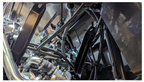
25. Locate the left (drivers side) intercooler bracket. Aluminum with "DLP" in the middle. Install the narrow side of the bracket over the larger of the two block-off plates. Again, leave these two fasteners as loose as possible until the final steps of installing the intercooler.
