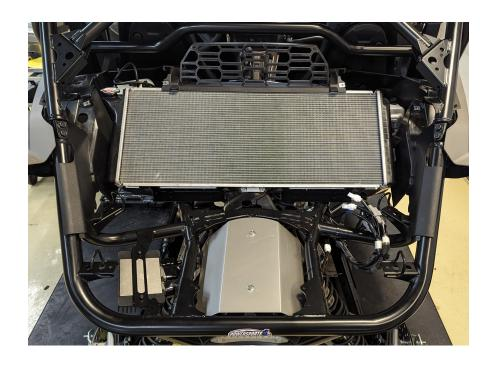
2. Locate the rear intake bracket. Remove the 8mm fastener connected to the intake housing and also the hose clamp attached the coolant line. Further down the coolant line is another hose clamp attached to the frame. Remove that fastener too. Both of these hose clamps will be reinstalled at a later time. With the coolant line free from the frame, use the drain port pictured below, and drain the coolant from the radiator.
