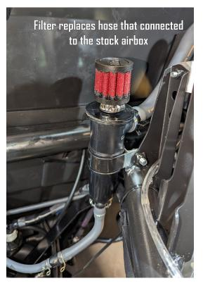
8. Loosen the intake clamps on the throttle bodies, unplug the intake air temp sensor, and remove the hose for the idle / air valve (this will be connected to the intercooler). Remove the intake box.
