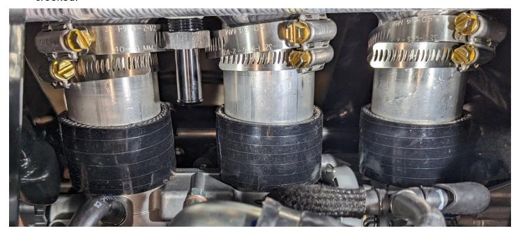
33. Once the intercooler is fully seated and couplers even, position the clamps. You want the clamps positioned as seen below. You want a small amount of silicone on the outside of each clamp. Otherwise the coupler will squish in causing a leak. Also make sure none of the clamps are interfering with the throttle.
